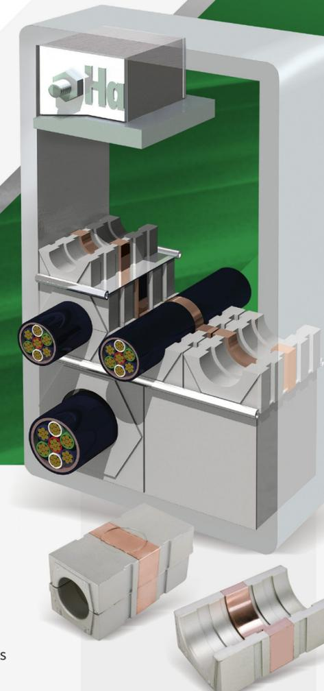
Stray signal/noise cannot pass through the conductive EMC and pass to earth. Tolerant and filler blocks have a cable range of 3mm to 100mm and are coated with a high conductive material. Copper tape provides high conductive path from cable screen to earth. Frame zinc plated or stainless steel to allow conductivity from blocks to earth. Simple preparation of cable and assembly of system without modification of insert blocks onsite.
